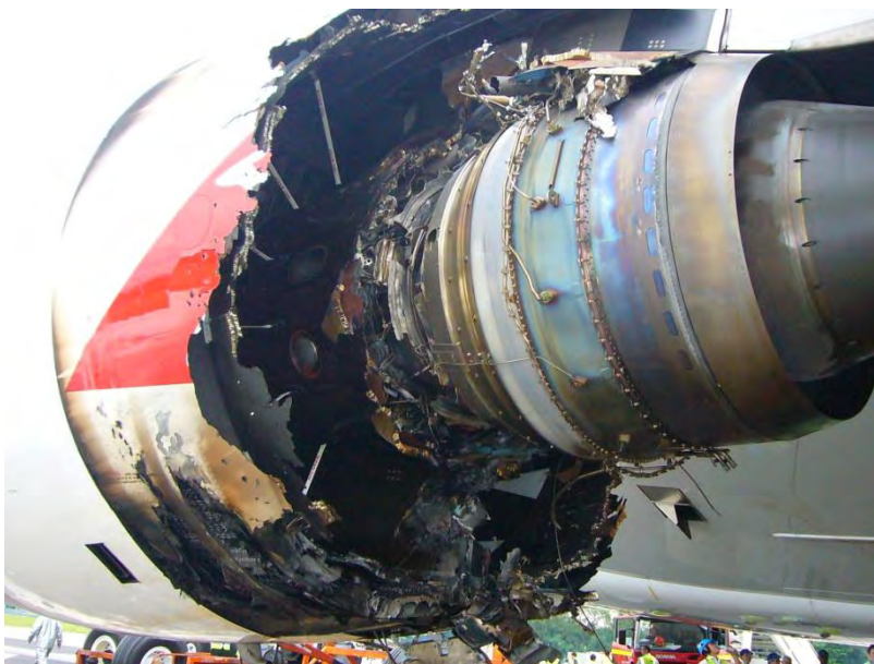
Figure 7: Damage to the No 2 engine
