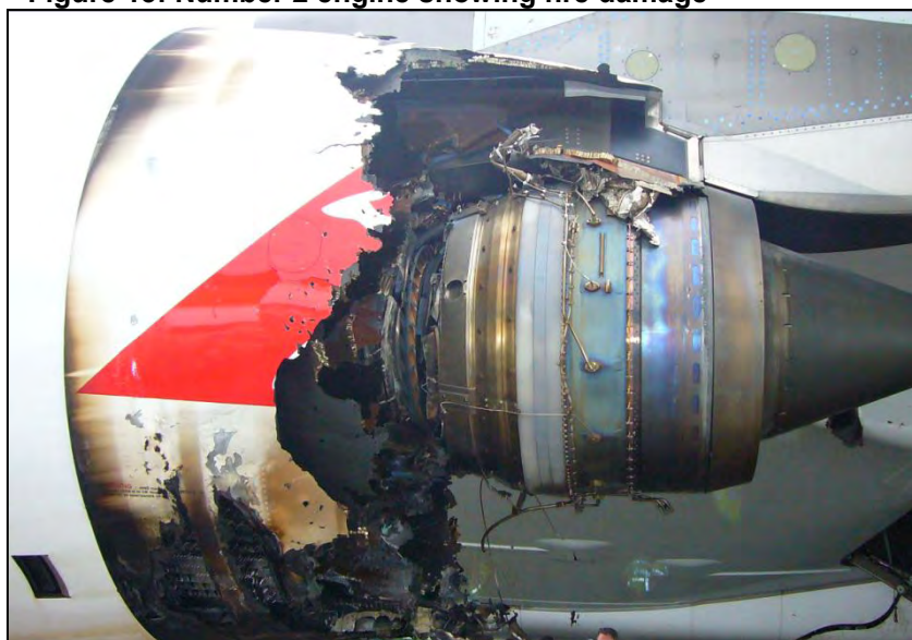
Figure 13: Number 2 engine showing fire damage
