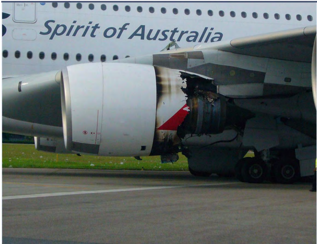
Figure 1: VH-OQA showing the damaged No 2 engine
